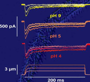
Voltage clamp recordings of mechanically-induced receptor current in a VS-3 neuron exposed to extracellular pH 9, pH 5, and pH 4. The neuron was clamped at a holding potential of -80 mV, the cell’s resting potential at extracellular pH 9. The lower traces show the deflection of the stimulator.
