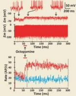
VS-3 neuron response to electrical pseud V>-3 neuron response to electrical pseudorandom noise stimulation is shown with and without action potentials (AP). Upper traces show the spikes before and after octopamine application on a different scale. Octopamine was ejected introhoretically at the time indicated. The lower traces show the AP firing rate from the recording above (red) and the AP rate of a control recording from the same neuron without octopamine application (blue).
